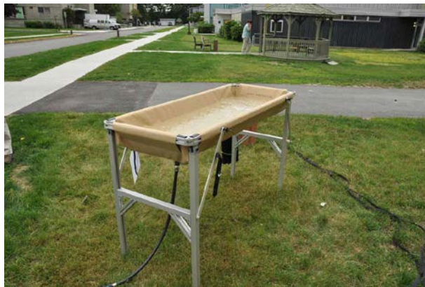
Figure 2-3: Arm Immersion Cooling System. To use, Soldiers Place their Forearms in the Cool Water, Covering the Area from the Fingers to the Elbow.
